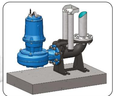
This is the most convenient solution for fixed installations, because the pump can be easily and quickly extracted and repositioned in the tank, meaning the pump can be serviced and cleaned without having to empty the tank or unbolt any parts.
